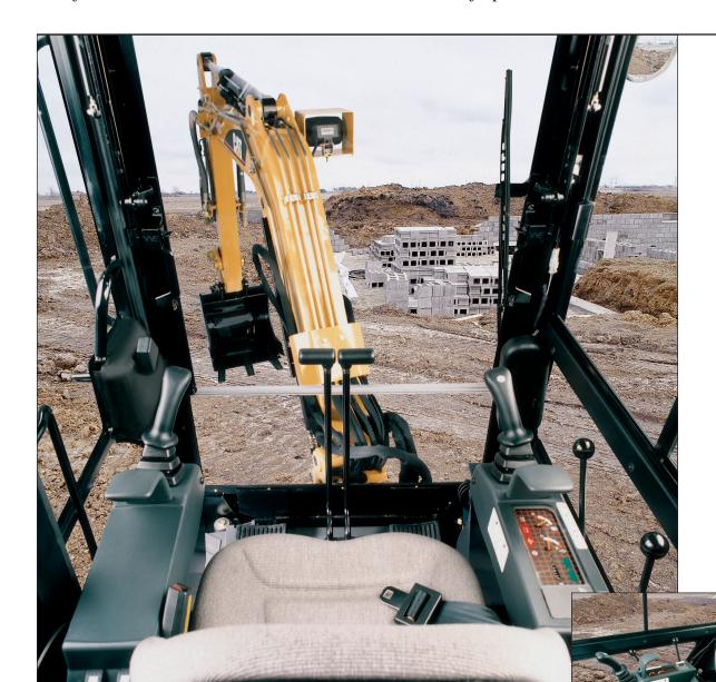
**Excellent viewing** to the work tool is possible with large windows and offset swing post. The curved hood and large rear glass give superior viewing to the rear. The easy-to-open front window, removable lower-front window and sliding right-side window offer excellent ventilation.
